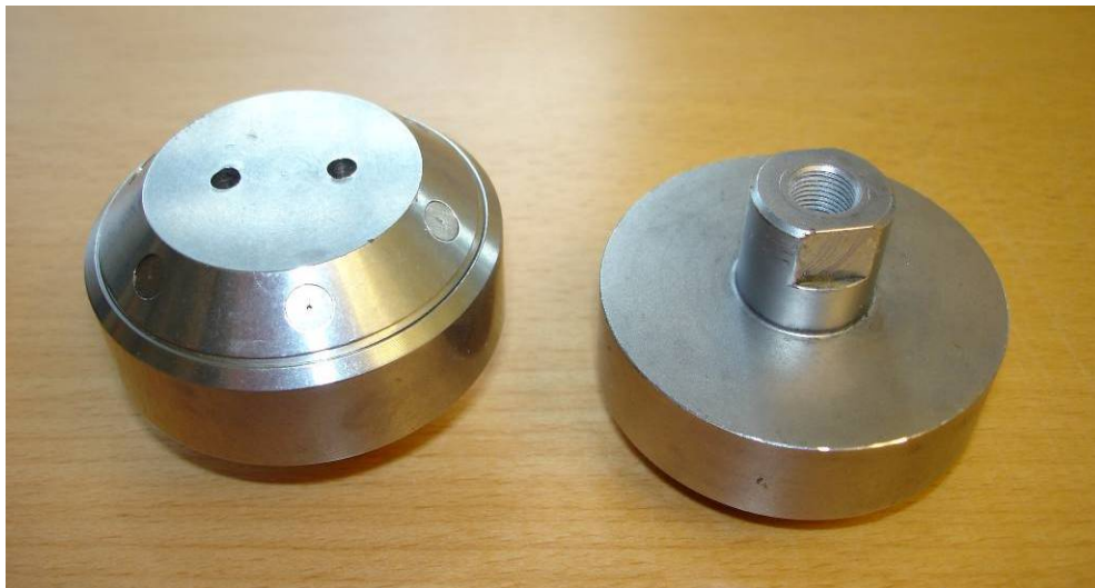
Figure 11 The ULTRA FOG nozzle used in the tests at SP in 1992.
